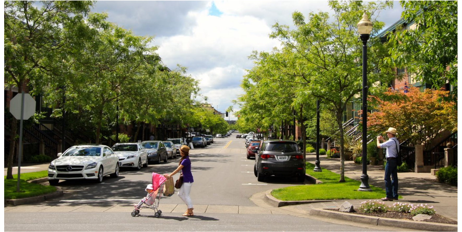
Landscaped Bulb-out Shortening Crosswalk Distance
